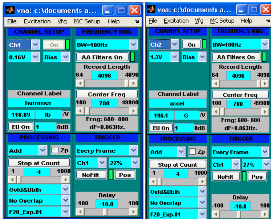
Figure 2.13 Channel 1 and channel 2 settings for Impact hammer testing
